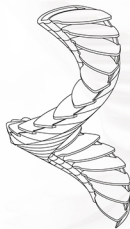
E.L.I.C.A. Diameter 210 cm; Riser: 17 cm ; Price single step: 220 Euro
